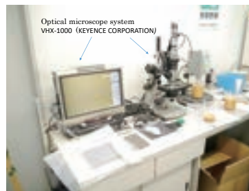
optical microscope for observation of the powders produced with L-8i
